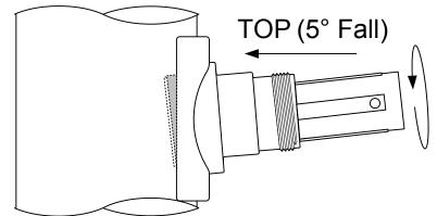
Insert Fixing Tool into Boss and turn NO MORE than three times anti-clockwise to tighten.
