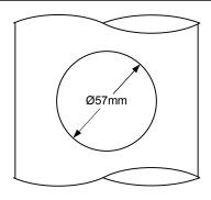
Cut 57mm hole in 110mm or 82mm pipe.
