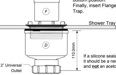
If a silicone sealant is used. it should be a neutral sealant and not an acetoxy sealant.
