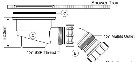
Connect Trap Outlet, *E*, to waste pipe, ensuring that the pipe is adequately supported. Test the installation.
