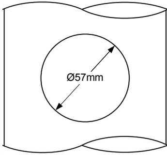
Cut 57mm hole in 110mm or 82mm pipe.
