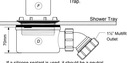
If a silicone sealant is used, it should be a neutral sealant and **not** an acetoxy sealant.
