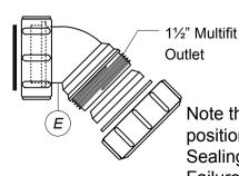
Note the order and position of the Sealing Washers. Failure to do so can result in water leakage.
