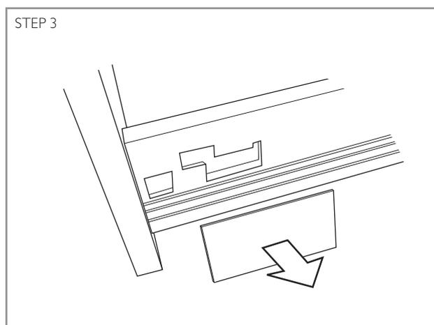
The drawer may require adjustment to ensure alignment. This is achieved with the adjustable runners. They are located at the front on the underside of the drawer. By rotating the wheel indicated in Step 3 vertical adjustment of the drawer can be made.
