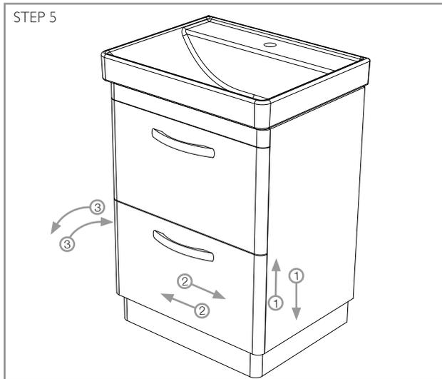
To make adjustment 1 (Up and Down) turn screw A (see Step 4)
