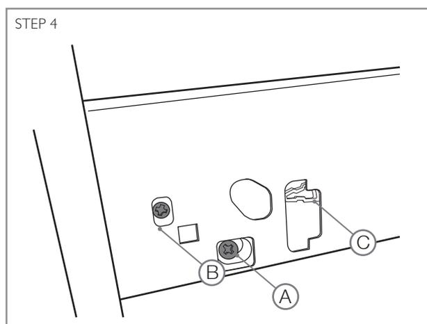
The drawers have a quick release function. The drawer is removed by squeezing the levers C on both of the runners and pulling the drawer forward.
